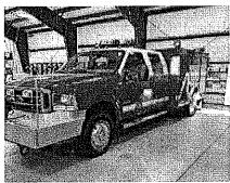
Rley 170 GPM Pump, 300 Gallon Tank, Foam System, Low Mi....
